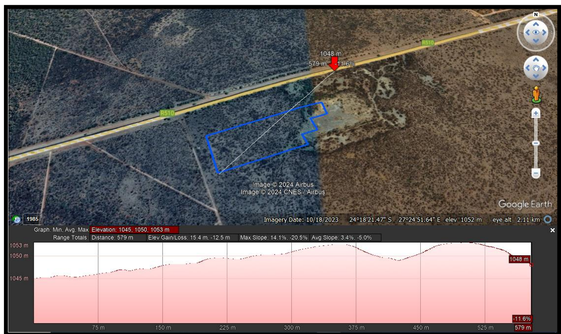
Figure 17: Elevation profile of the proposed mining footprint (Image obtained from Google Earth).
